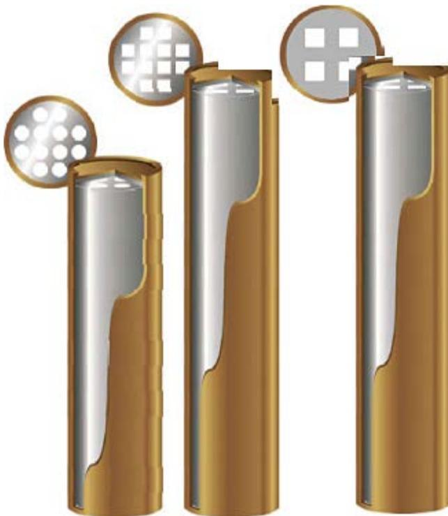
*Figure 1-1. Canister types for VVER, BWR and PWR spent fuel assemblies with 12, 12 and 4 assembly positions in each canister.*
